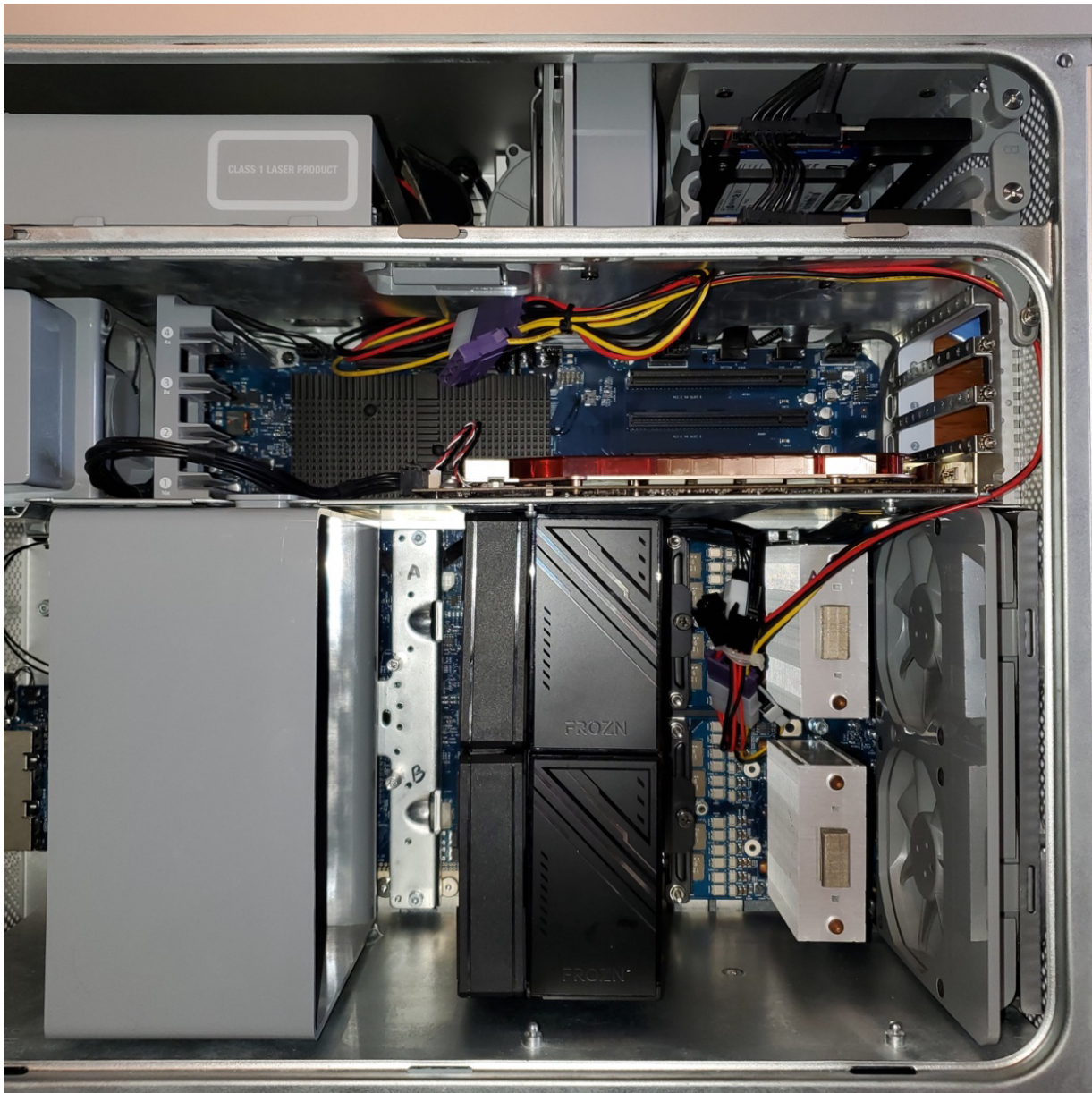
Finished air cooling modification of Power Mac G5 Quad Photo courtesy of MacRumors user Amishallan
