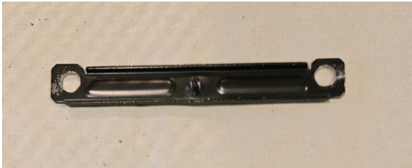
Front Mounting Bracket with Enlarged Holes
