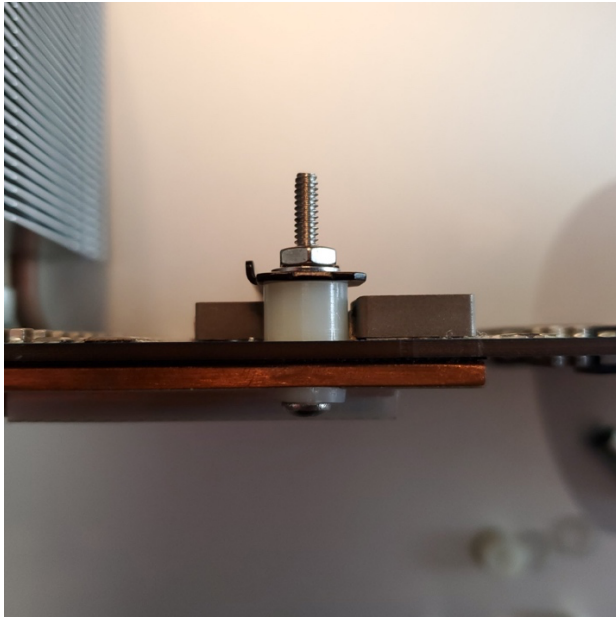
Back Mounting Hardware Screwed Down, Offset by Plastic Washer Photo courtesy of MacRumors user Amishallan
