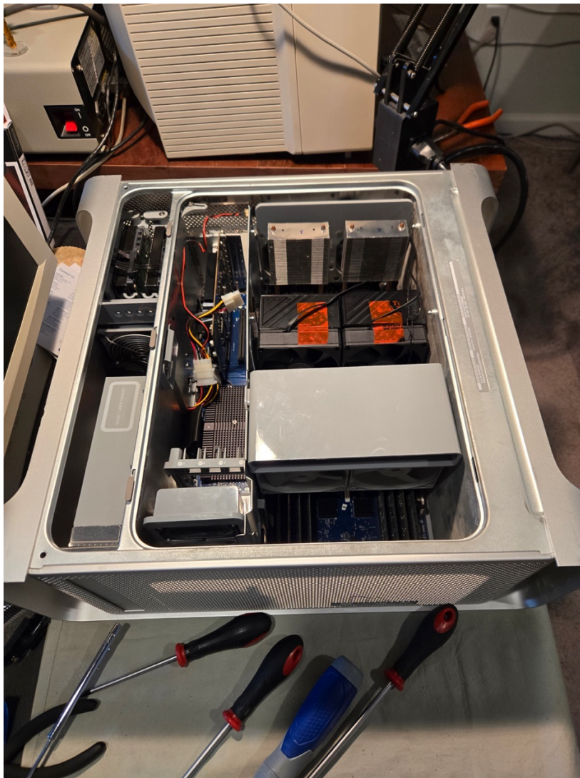
Fans attached to the FROZN A400 units
